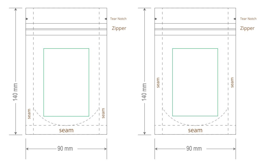
Green area is the bag area is the printing area, artwork with at most 2 colors for silkscreen printing. Note: In Silkscreen printing Text font size must be bigger than 11pt can be clearly printed.
