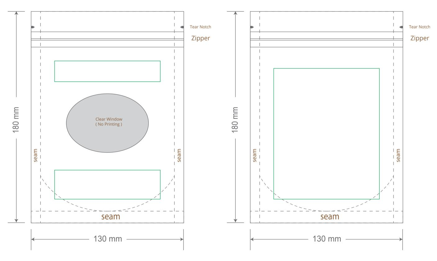
Green area is the bag area is the printing area, artwork with at most 2 colors for silkscreen printing. Note: In Silkscreen printing Text font size must be bigger than 11pt can be clearly printed.
