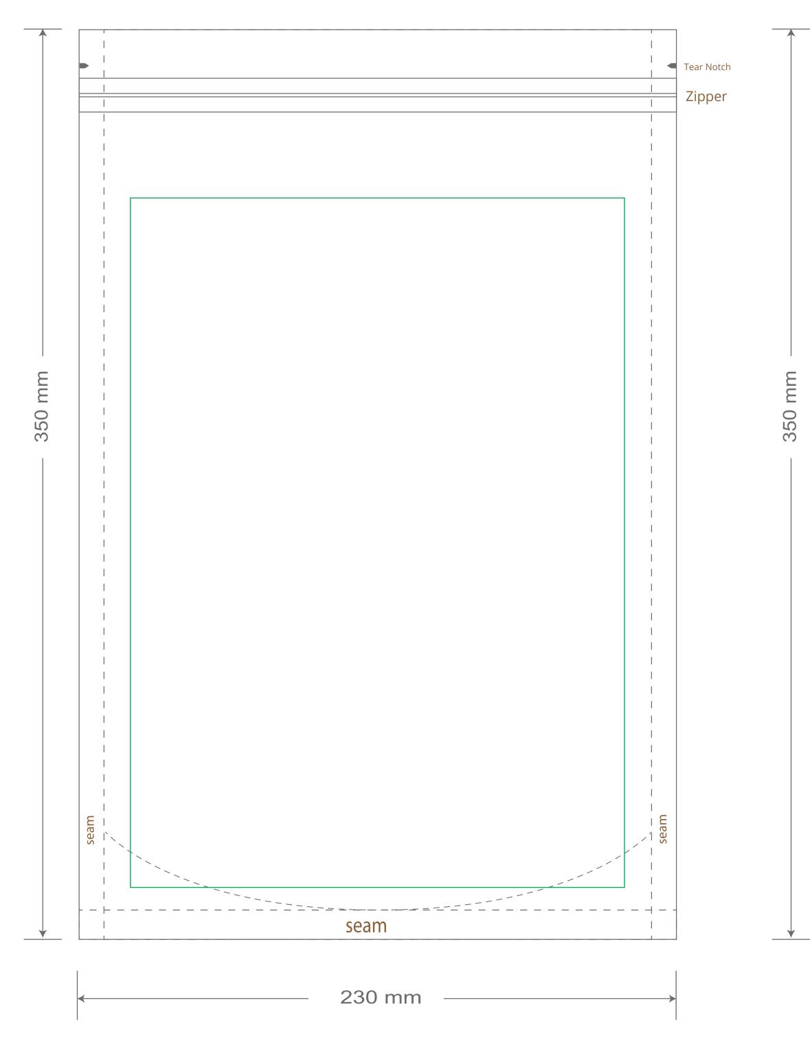
Green area is the bag area is the printing area, artwork with at most 2 colors for silkscreen printing. Note: In Silkscreen printing Text font size must be bigger than 11pt can be clearly printed.
